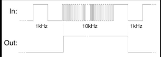
Create a circuit that can distinguish a 1kHz squarewave from a 10kHz squarewave
